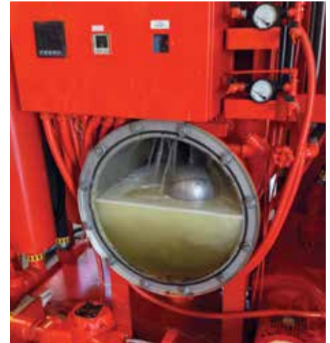
Vacuum dehydrator used to remove water contamination.
