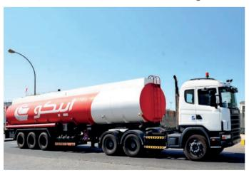
with a maximum 10ppm sulphur content. After six months of testing, they exceeded the initial objective and raised ODI to 35,000 km. Which met and exceed the project oil drain extension target.
